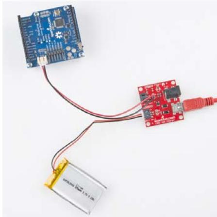
*You can use the "SYS OUT" header to power a 3.3V Arduino Pro. All while leaving your battery connected to the charger.*
