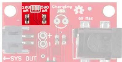
If you look *really* closely at that jumper, you may see a small trace connecting the middle pad to the *500mA*-labeled outer pad. As such, this board is **configured to deliver a 500mA current by default**.
