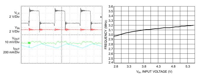
Figure 18. PWM Mode of Operation ( $V_{IN}$  = 3.6 V,  $V_{OUT}$  = 1.2 V,  $I_{OUT}$  = 300 mA, 25°C)
