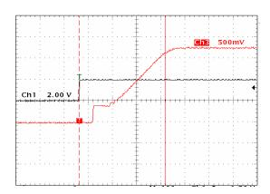
Figure 17. Soft Start Time (V<sub>IN</sub> = 3.6 V)
