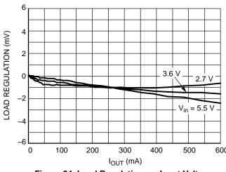
Figure 24. Load Regulation vs. Input Voltage (V<sub>OUT</sub> = 1.2 V, 25°C)
