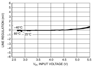
Figure 27. Line Regulation vs. Temperature (V<sub>OUT</sub> = 1.2 V, I<sub>OUT</sub> = 100 mA)
