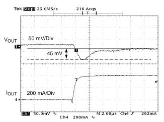
Figure 33. Load Transient Response ( $V_{IN}$  = 3.6 V,  $V_{OUT}$  = 1.2 V, 0 mA to 400 mA step)
