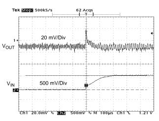
Figure 31. Line Transient Response (V<sub>IN</sub> step = 600 mV, V<sub>OUT</sub> = 1.2 V)
