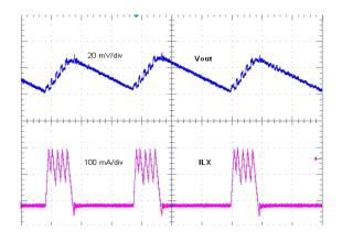
Figure 13. Step Down Converter PFM Mode Operation
