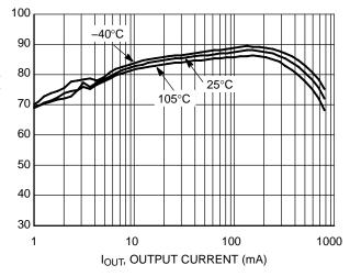
Figure 6. Efficiency vs. Output Current  $(V_{OUT} = 1.8 \text{ V}, V_{IN} = 3.6 \text{ V})$
