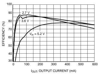
Figure 20. Efficiency vs. Output Current (V<sub>OUT</sub> = 1.2 V, 25°C)
