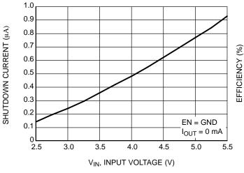
Figure 5. Shutdown Current vs. Supply Voltage
