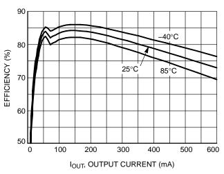
Figure 21. Efficiency vs. Output Current (V<sub>OUT</sub> = 1.2 V, V<sub>IN</sub> = 3.6 V)
