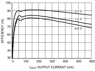
Figure 22. Efficiency vs. Output Current (V<sub>IN</sub> = 3.6 V, 25°C)
