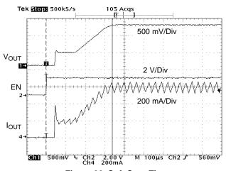
Figure 30. Soft Start Time ( $V_{IN}$  = 3.6 V,  $V_{OUT}$  = 1.2 V,  $I_{OUT}$  = 600 mA)
