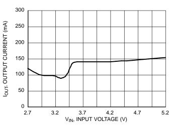
Figure 12. PFM/PWM Threshold vs. Input Voltage
