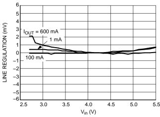
Figure 26. Line Regulation vs. Output Current (V<sub>OUT</sub> = 1.2 V, 25°C)
