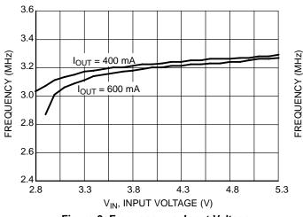
Figure 9. Frequency vs. Input Voltage
