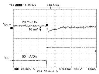
Figure 32. Load Transient Response ( $V_{IN}$  = 3.6 V,  $V_{OUT}$  = 1.2 V, 0 mA to 95 mA step)
