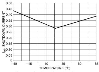
Figure 28. Shutdown Current vs. Temperature (V<sub>OUT</sub> = 3.6 V)
