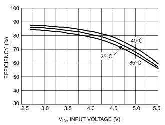
Figure 23. Efficiency vs. Input Current (V<sub>OUT</sub> = 1.2 V, I<sub>OUT</sub> = 100 mA)
