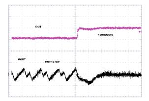
Figure 16. Load Transient Response Between PFM and PWM Operation (100 mA to 200 mA)
