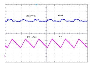
Figure 14. Step Down Converter PWM Mode Operation
