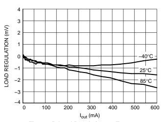
Figure 25. Load Regulation vs. Temperature (V<sub>IN</sub> = 3.6 V, V<sub>OUT</sub> = 1.2 V)
