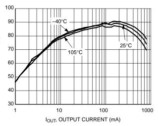
Figure 8. Efficiency vs. Output Current ( $V_{OUT} = 2.0 \text{ V}, V_{IN} = 3.6 \text{ V}$ )
