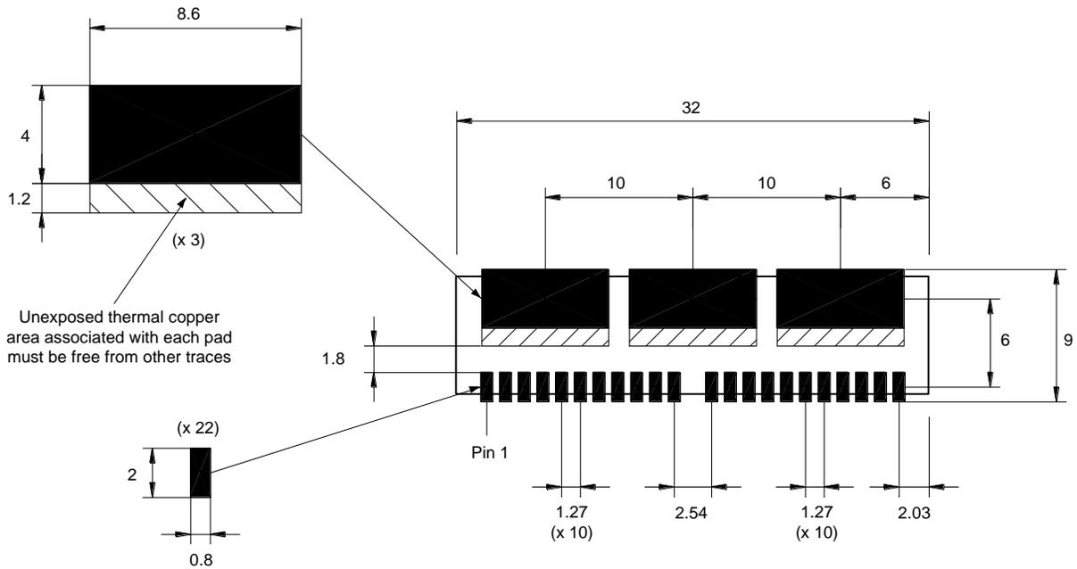
Figure 58: Recommended PCB Layout for Multilayer PCBs
