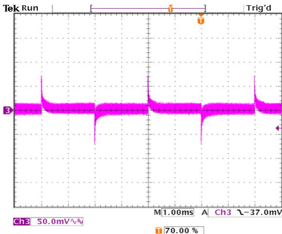
Figure 48. Transient Response with Regulation set to 1.89 mv/A.
