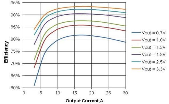
Figure 7: Efficiency vs. Output voltage for converter DP7130, with 30A load, input voltage at 8, 12 and 14V, at Ta = 25 °C.
