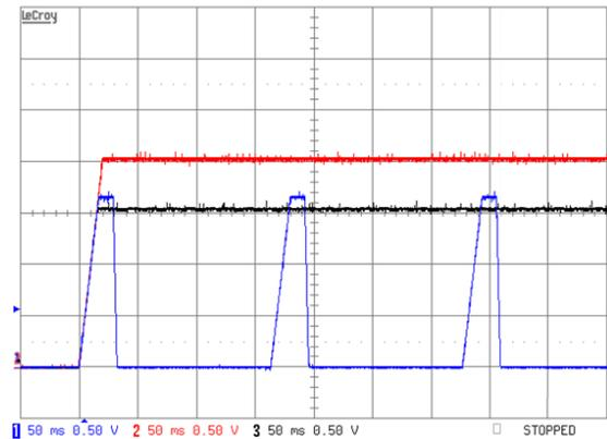
Figure 36 shows a scope capture an actual system when undervoltage error detection is set to not propagate.
