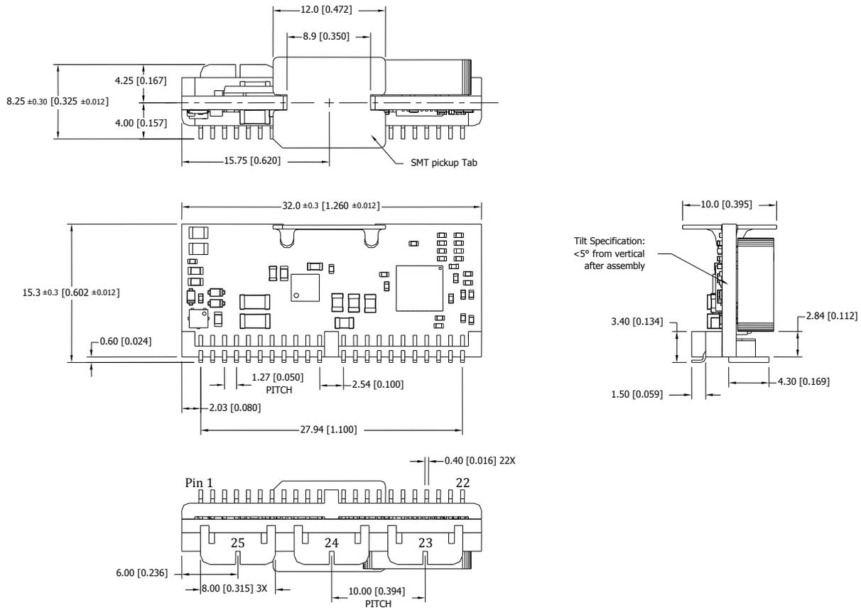
Figure 56: Pinout Diagram (Bottom View)
