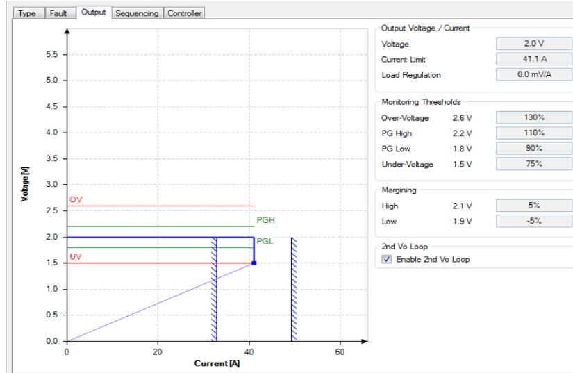
Note that the GUI shows the effect of setting PG, OV and UV limits as both values and graphical limit bars. Vertical hashed lines are error bars for the Overcurrent (OC) limit.
