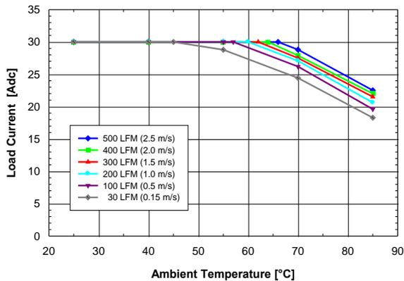
Figure 4: Available output power vs. ambient air temperature and airflow rates for converter DP7130G mounted horizontally with air flowing from pin 1 to pin 22, MOSFET temperature  $\leq 125^\circ\text{C}$ ,  $V_{in} = 12\text{ V}$ .
