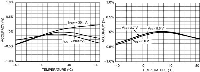
Figure 9. Output Voltage Accuracy vs. Temperature (V<sub>IN</sub> = 3.6 V, V<sub>OUT</sub> = 1.2 V)
