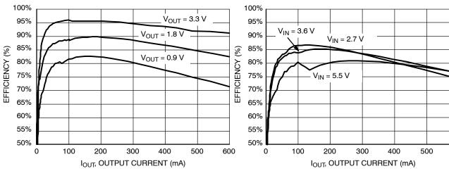
Figure 11. Efficiency vs. Output Current  $(V_{IN} = 3.6 \text{ V}, T_A = 25^{\circ}\text{C})$
