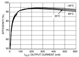
Figure 29. Efficiency vs. Output Current (V<sub>IN</sub> = 5.0 V, V<sub>OUT</sub> = 3.9 V)
