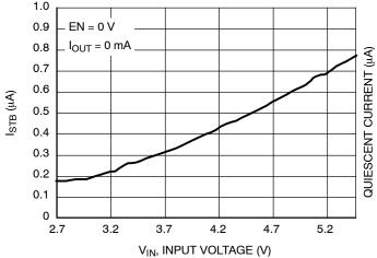
Figure 7. Shutdown Current vs. Supply Voltage
