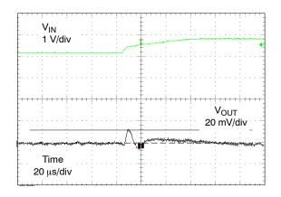
Figure 19. 3.0 V to 3.6 V Line Transient (Risetime = 50  $\mu$ s, V<sub>OUT</sub> = 1.2 V, I<sub>OUT</sub> = 100 mA, T<sub>A</sub> = 25°C)
