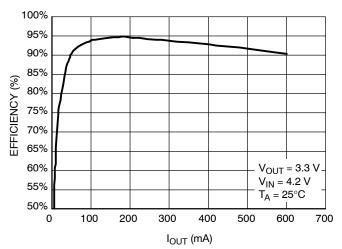
Figure 3. Efficiency vs. Output Current
