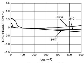
Figure 21. Load Regulation (V<sub>IN</sub> = 3.6 V, V<sub>OUT</sub> = 1.2 V)
