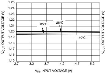
Figure 17. Line Regulation (V<sub>OUT</sub> = 1.2 V, I<sub>OUT</sub> = 100 mA)
