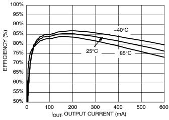
Figure 13. Efficiency vs. Output Current (V<sub>IN</sub> = 3.6 V, V<sub>OUT</sub> = 1.2 V)
