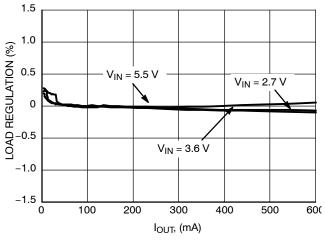
Figure 22. Load Regulation (V<sub>OUT</sub> = 1.2 V, T<sub>A</sub> = 25°C)
