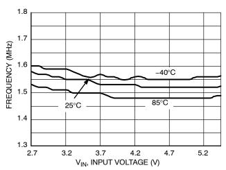
Figure 14. Switching Frequency vs. Input Voltage (V<sub>OUT</sub> = 1.2 V, I<sub>OUT</sub> = 300 mA)
