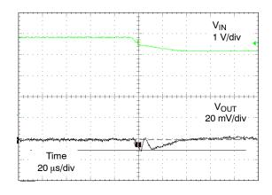
Figure 20. 3.6 V to 3.0 V Line Transient (Risetime = 50  $\mu$ s, V<sub>OUT</sub> = 1.2 V, I<sub>OUT</sub> = 100 mA, T<sub> $\Delta$ </sub> = 25°C)
