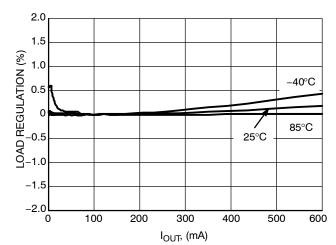
Figure 30. Load Regulation (V<sub>IN</sub> = 5.0 V, V<sub>OUT</sub> = 3.9 V)
