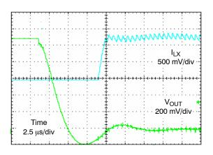
Figure 16. Short-Circuit Protection  $(V_{IN} = 3.6 \text{ V}, V_{OUT} = 1.2 \text{ V})$
