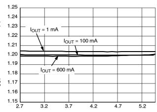
Figure 18. Line Regulation (V<sub>OUT</sub> = 1.2 V, T<sub>A</sub> = 25°C)
