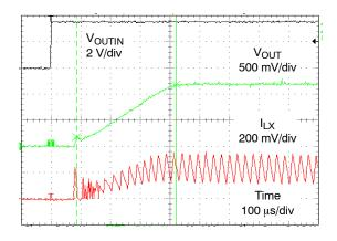
Figure 15. Typical Soft-Start (V<sub>IN</sub> = 3.6 V, V<sub>OUT</sub> = 1.2 V, I<sub>OUT</sub> = 250 mA)
