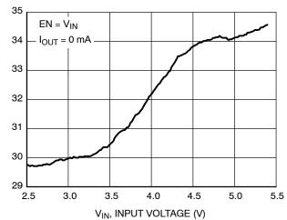
Figure 8. Quiescent Current PFM No Switching vs. Supply Voltage
