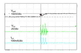
Figure 28. PFM Mode Switching Waveform (V<sub>IN</sub> = 3.6 V, V<sub>OUT</sub> = 1.2 V, I<sub>OUT</sub> = 0 mA)
