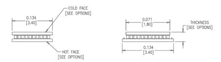
Ceramic material 96% Alumina ceramics Solder construction: 138°C BiSn
