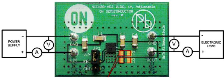
Please solder feedback resistors to program the output voltage. The resistors should be 1206 SMD type. \*During the tests please leave the JP1 disconnected
