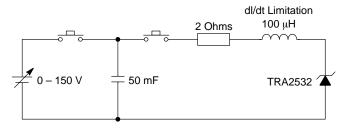
Figure 11. Load Dump Test Circuit
