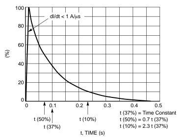
Figure 12. Load Dump Pulse Current
