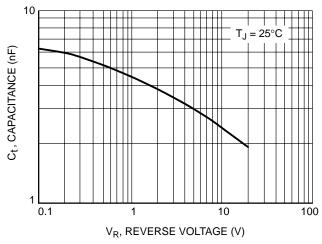
Figure 2. Typical Reverse Capacitance
