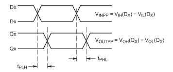
Figure 3. AC Reference Measurement
