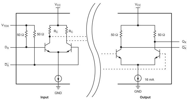
Figure 5. CML Input and Output Structure
