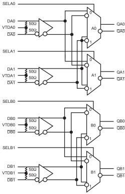
Figure 1. Functional Block Diagram
