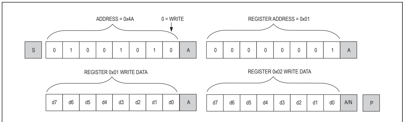
Figure 11. Format for Writing to Multiple Registers
