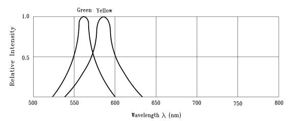
Fig.1 RELATIVE INTENSITY VS. WAVELENGTH
