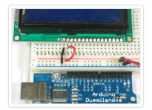
Next we'll connect up the backlight for the LCD. Connect pin 16 to ground and pin 15 to +5V. On the vast majority of LCDs (including ones from Adafruit) the LCD includes a series resistor for the LED backlight.
