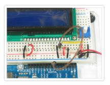
Next is the **RS** pin #4. We'll use a brown wire to connect it to Arduino's digital pin #7.
