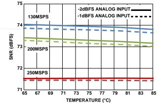
FIGURE 27. TYPICAL SNR PERFORMANCE vs TEMPERATURE, DEVICE CALIBRATED AT +85°C, f<sub>IN</sub> = 105MHz
