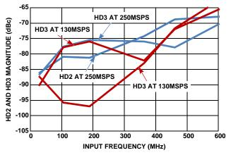
FIGURE 6. HD2 AND HD3 vs f<sub>IN</sub>
