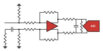
FIGURE 32. DIFFERENTIAL AMPLIFIER INPUT
