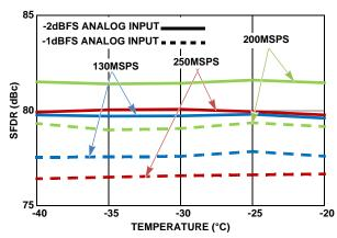
FIGURE 24. TYPICAL SFDR PERFORMANCE vs TEMPERATURE, DEVICE CALIBRATED AT -40°C, f<sub>IN</sub> = 105MHz
