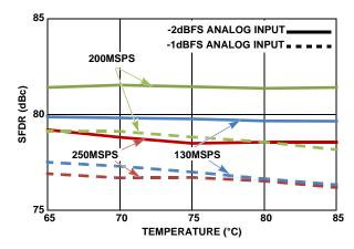
FIGURE 28. TYPICAL SFDR PERFORMANCE VS TEMPERATURE, DEVICE CALIBRATED AT +85°C, f<sub>IN</sub> = 105MHz
