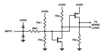
FIGURE 47. TRI-LEVEL DIGITAL INPUTS
