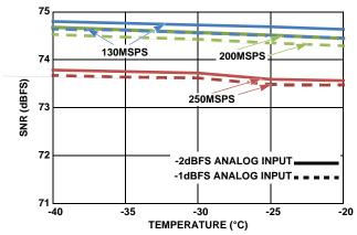
FIGURE 23. TYPICAL SNR PERFORMANCE vs TEMPERATURE, DEVICE CALIBRATED AT -40°C, f<sub>IN</sub> = 105MHz
