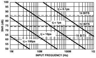
FIGURE 34. SNR vs CLOCK JITTER
