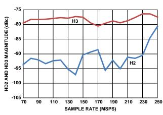
FIGURE 10. HD2 AND HD3 vs f<sub>SAMPLE</sub>
