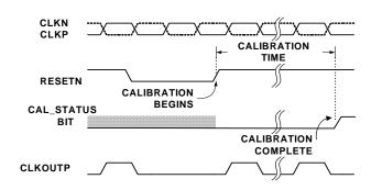
FIGURE 22. CALIBRATION TIMING
