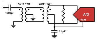
FIGURE 30. TRANSFORMER INPUT FOR GENERAL PURPOSE APPLICATIONS
