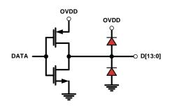
FIGURE 50. CMOS OUTPUTS
