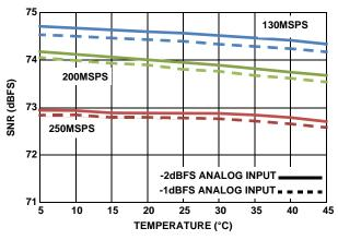
FIGURE 25. TYPICAL SNR PERFORMANCE vs TEMPERATURE, DEVICE CALIBRATED AT +25°C, f<sub>IN</sub> = 105MHz
