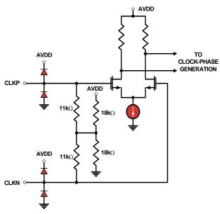
FIGURE 46. CLOCK INPUTS
