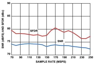
FIGURE 9. SNR AND SFDR vs f<sub>SAMPLE</sub>
