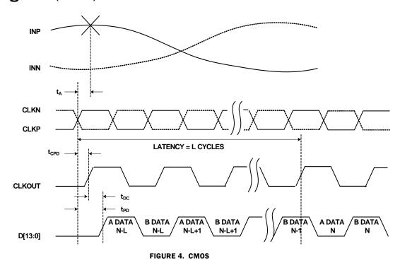
**Switching Specifications** Boldface limits apply over the operating temperature range, -40 °C to +85 °C.
