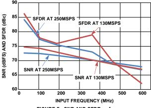
FIGURE 5. SNR AND SFDR vs fin
