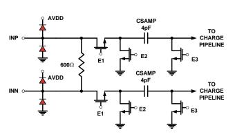
FIGURE 45. ANALOG INPUTS
