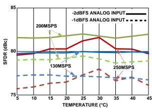
FIGURE 26. TYPICAL SFDR PERFORMANCE vs TEMPERATURE, DEVICE CALIBRATED AT +25°C, f<sub>IN</sub> = 105MHz
