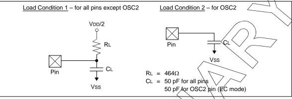
TABLE 12-7: CAPACITIVE LOADING REQUIREMENTS ON OUTPUT PINS
