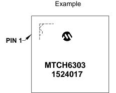
64-Lead TQFP (10x10x1 mm)
