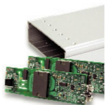
Standard Xgen product options include: Conformal Coating, Low Acoustic noise, Low Leakage Current, Connector, Cabling & Mounting options, Thermal Signals and Reverse Fans. See section 4.10 for more details.
