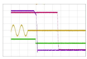
Figure 8. Turn-Off AC Line 230 VAC, half load (20 ms/div)
