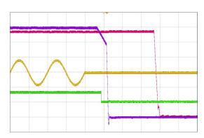
Figure 6 - Turn-Off AC Line 230 VAC, full load (10 ms/div) CH1: Vin (400 V/div) CH2: PWOK\_H (5 V/div) CH3:  $V_1$  (2 V/div) CH4:  $V_{SB}$  (2 V/div)
