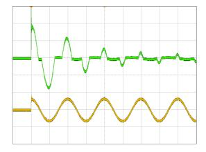
Figure 4. Inrush current, V<sub>in</sub> = 230 Vac, 90° CH1: V<sub>in</sub> (500 V/div), CH2: I<sub>in</sub> (10 A/div
