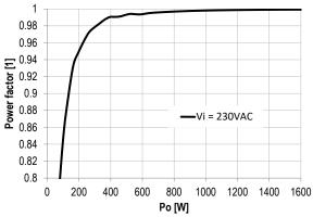
Figure 3. Power factor vs. Load current
