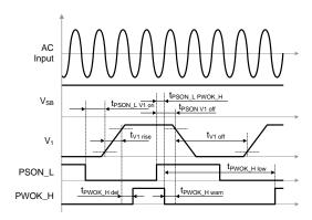
Figure 27. PSON\_L turn-on/off timing
