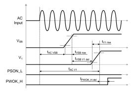
Figure 24. AC turn-on timing
