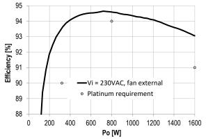
Figure 2. Efficiency vs. Load current (ratio metric loading)
