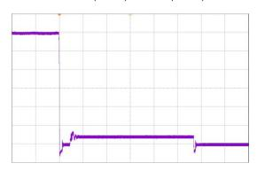
Figure 10. Short circuit on V1 (10 ms/Div) CH3: V<sub>1</sub> (2 V/div)
