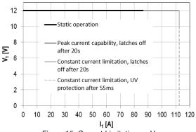
Figure 15. Current Limitation on V<sub>1</sub> at V<sub>i</sub> = 90 ... 140 VAC
