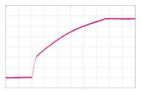
Figure 9. Turn-On AC Line 230 VAC, full load (2 ms/div) CH4: V<sub>SB</sub> (2 V/div)
