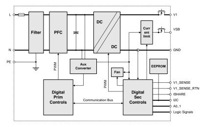
Figure 1. PET1600-12-074NA Block Diagram
