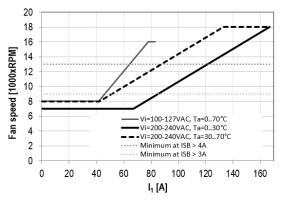
Figure 34. Fan speed vs. main output load
