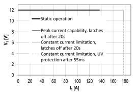
Figure 16. Current Limitation on  $V_1$  at  $V_1 = 180 \dots 264 \text{ VAC}$
