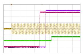
Figure 5. Turn-On AC Line 230 VAC, full load (200 ms/div) CH1: Vin (400 V/div) CH2: PWOK\_H (5 V/div) CH3: V<sub>1</sub> (2 V/div) CH4: V<sub>SB</sub> (2 V/div)
