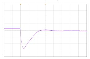
Figure 11. Load transient V<sub>1</sub>, 133A to 67A (1 ms/div) CH3: V<sub>1</sub> (2 V/div) CH4: V<sub>SB</sub> (2 V/div)
