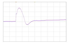
Figure 12. Load transient  $V_1$ , 67 A to 133 A (1 ms/div) CH3:  $V_1$  (200 mV/div)
