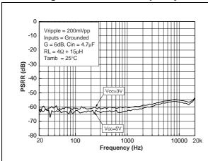
Figure 15. PSRR vs. frequency
