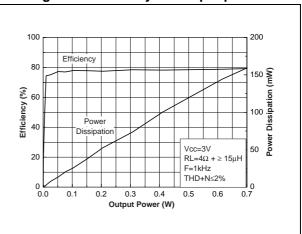
Figure 10. Efficiency vs. output power
