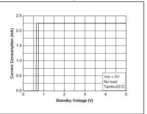
Figure 6. Current consumption vs. standby voltage
