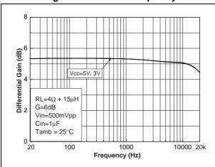
Figure 49. Gain vs. frequency
