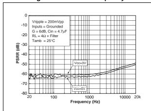
Figure 17. PSRR vs. frequency
