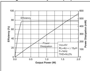
Figure 9. Efficiency vs. output power
