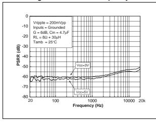
Figure 19. PSRR vs. frequency
