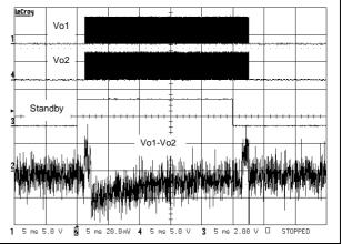
Figure 58. Startup & shutdown time  $V_{CC}$  = 3 V, G = 6 dB,  $C_{in}$  = 100 nF (5 ms/div)
