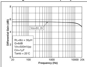
Figure 53. Gain vs. frequency
