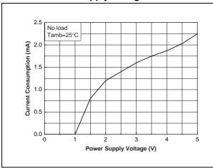
Figure 5. Current consumption vs. standby voltage
