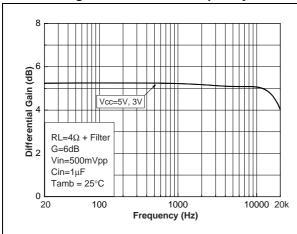
Figure 51. Gain vs. frequency
