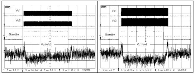
Figure 60. Startup & shutdown time  $V_{CC} = 3 \text{ V}$ , G = 6 dB, No  $C_{in}$  (5 ms/div)
