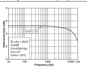
Figure 50. Gain vs. frequency
